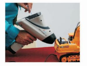
Cd in this toy is RoHS incompliant: Content of Cd is 140.8ppm>100ppm CBr in this toy is Non-halogen compliant: Content of Br is 808ppm<1500ppm
